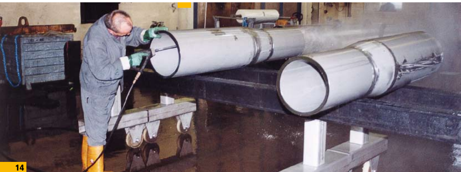
Fig. 25: Spray pickling of a prefabricated piping component
