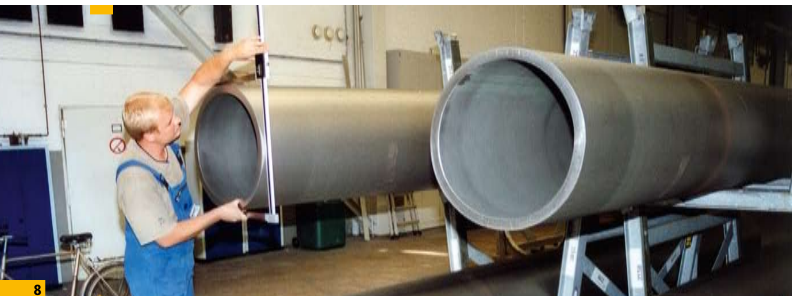
Fig. 8: Superduplex pipes, 609.6 × 38.89 mm
