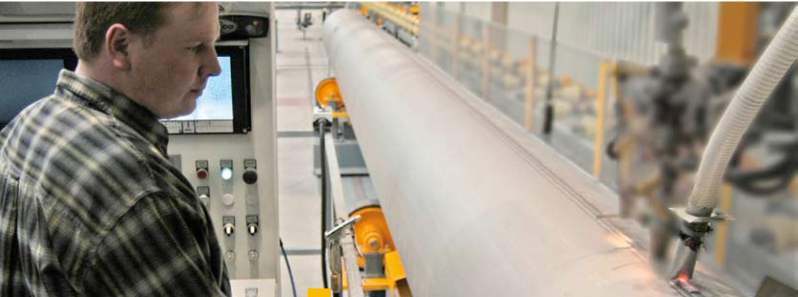
Fig. 13: Welding of superduplex pipes in 12 metre lengths without circumferential weld
