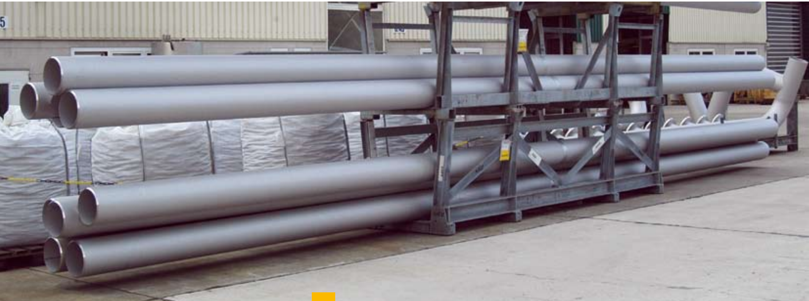
Fig. 36: For the AFAM project, 12 m lengths of pipe in duplex material were produced
