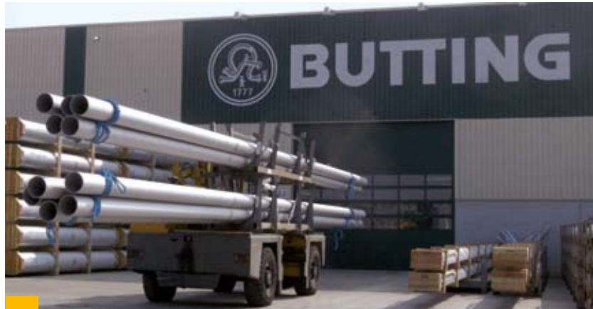
Fig. 34: Duplex pipes in 18 m lengths are used in the exploitation of Germany's largest natural gas field – Mittelplate
