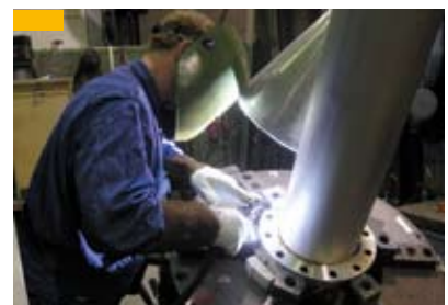
Fig. 16: Welding of BUTTING riser pipes made of superduplex for the oil and gas industry
