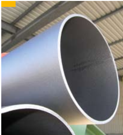
Fig. 24: Products made of special materials are blasted to reduce pickling times
