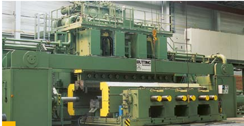
Fig. 20: Hydraulic calibration of pipes up to 12 metres enabling most stringent tolerances on the entire pipe body
