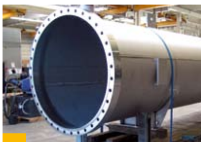
Fig. 30: Jacketed vessel in duplex for Shell in OD 1,521 x 10 mm
