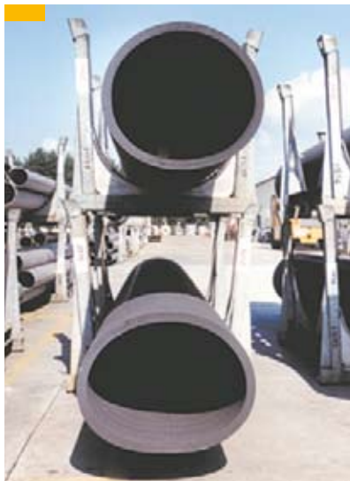
Fig. 19: Heat treated superduplex pipes waiting for calibration
