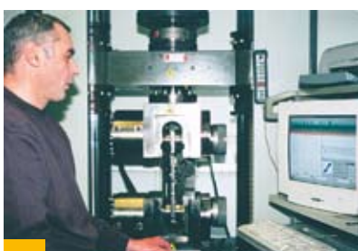
Fig. 28: Burkhard Hirtz at tensile test with microstrain measurement
