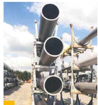
Fig. 6: Superduplex pipes after heat treatment
