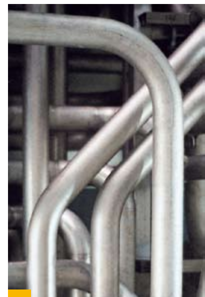
Multiple bends are produced at BUTTING using a mandril
