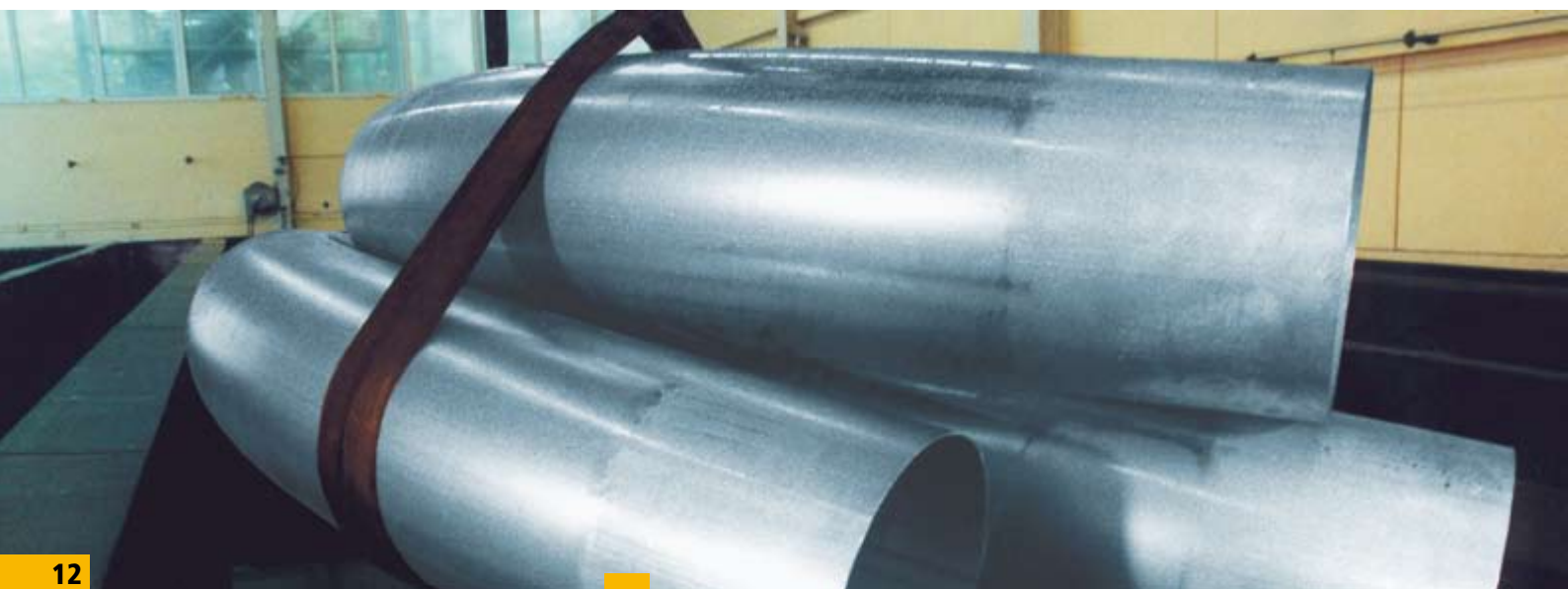
Special pickling plant for piggable elbows with long radii to guarantee the required surface quality
