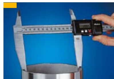
Measurement of the pipe inside diameter including the ovality
