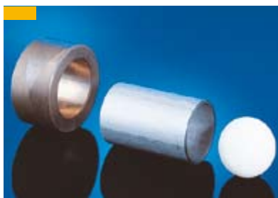
Testing during production using an outside gage and a ball for the inside
