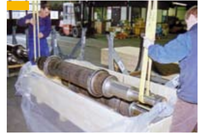
Seaworthy packing for BUTTING HeRo® (furnace roller)
