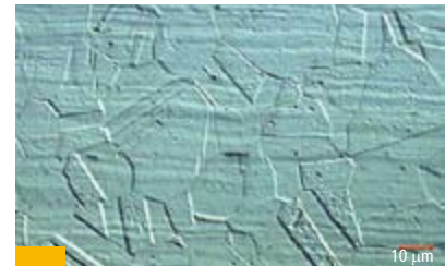
Macrograph of non titanium stabilized material
