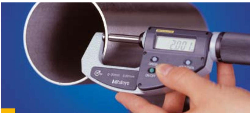
Measurement of wall thickness
