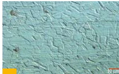
Macrograph of titanium stabilized material
