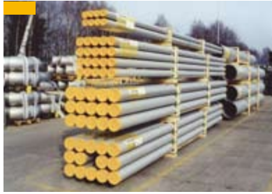
Piggable pipes ready for shipment with plastic end caps
