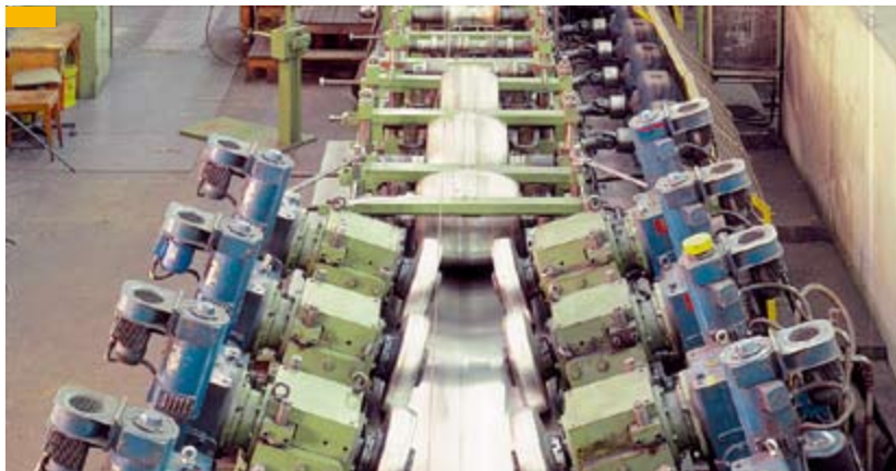
Continuous pipe production line for pipes from coil
