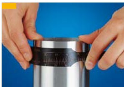
Measurement of the circumference to determine the inside diameter
