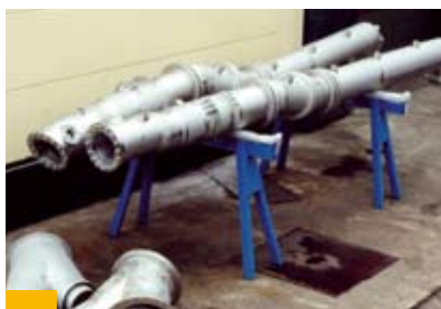
Mufflers for HDW Kiel after cleaning in the pickling bath
