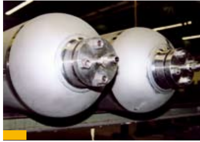
Pressure vessels for emergency air systems in submarines
