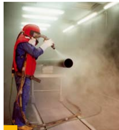
Glass marble peening improves the surface properties
