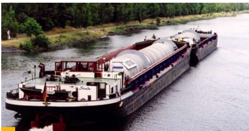
By ship: transport of blow tanks for the pulp mill in Stendal
