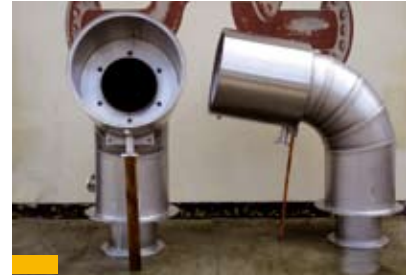
Sea water-cooled exhaust manifolds for a clean-up ship
