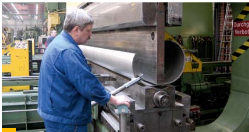
III. 15: Production of a pipe by forming a plate
