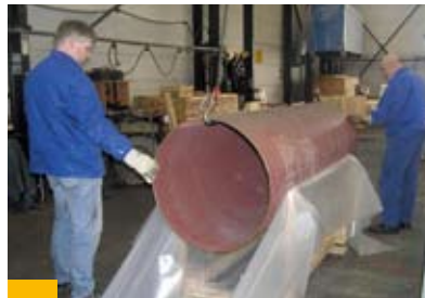
III. 38: Pipes in material 1.6780/HY 80 packaged for a specific project
