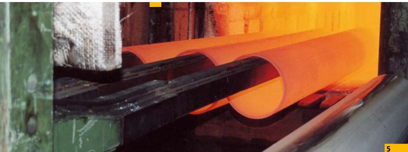
III. 5: Duplex pipes immediately after heat treatment
