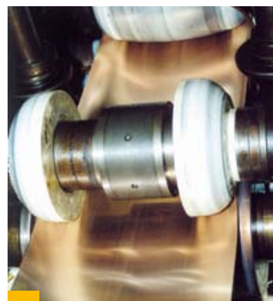
III. 16: Continuous forming of the coil by cold-forming
