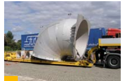
III. 41: Heavy transport of a segment elbow for a flood control reservoir
