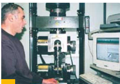
III. 28: Burkhard Hirtz at tensile test with microstrain measurement
