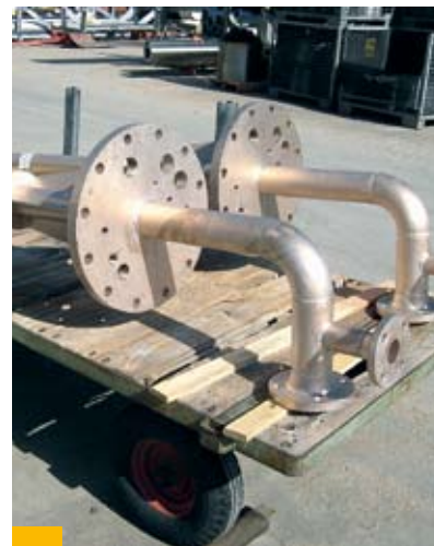
III. 20: Producing fittings for pipework systems for well equipment from a copper-nickel alloy
