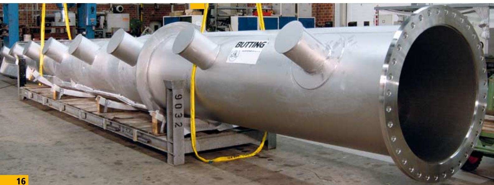
III. 32: Central pipe for an injection stage in the world's largest exhaust gas scrubbing system in Canada
