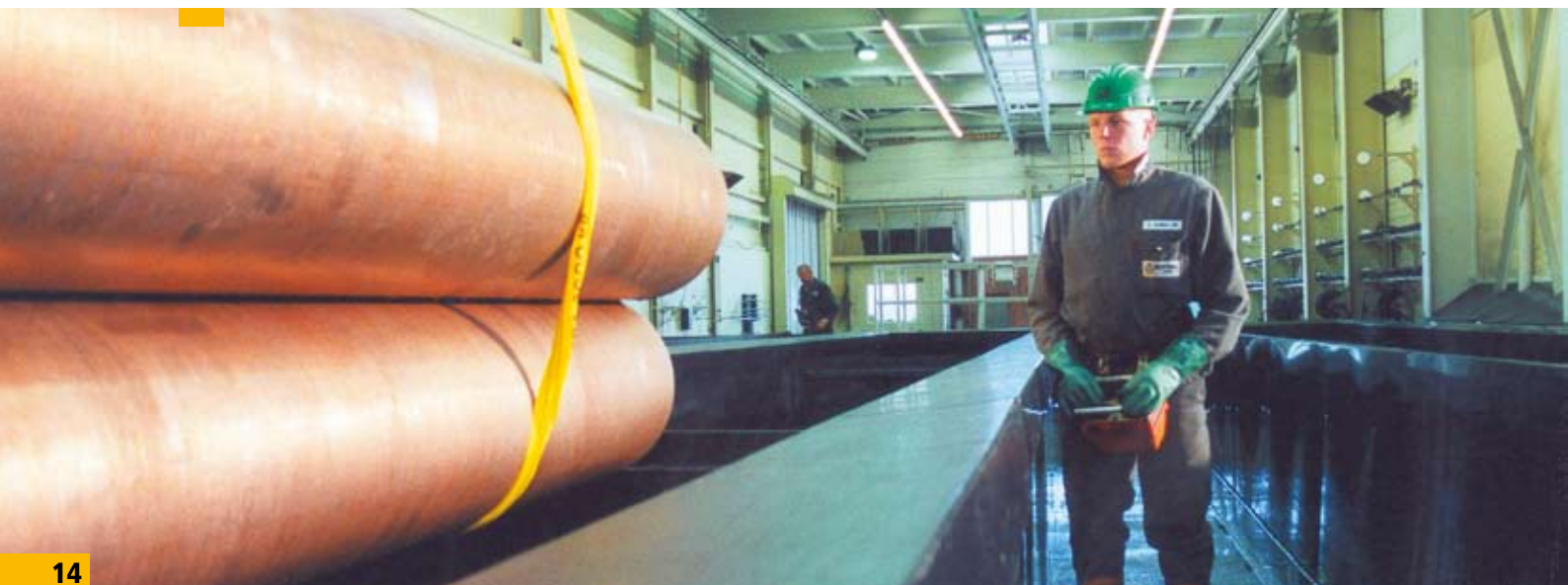
III. 26: Full-body pickling of pipes in a copper-nickel alloy using adequate pickling media
