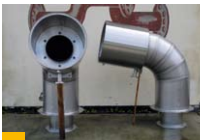
III. 33: Seawater-cooled flue gas manifold for a hazardous material accident ship in material 1.4565
