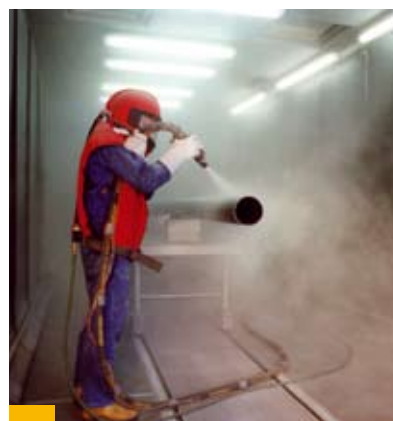
Our products can be blasted with glass beads to meet visual requirements
