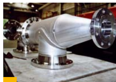
Pipe component with reinforced branch in Superduplex material for well construction
