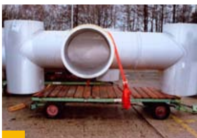
Prefabrication at the factory improves the quality of the pipe
