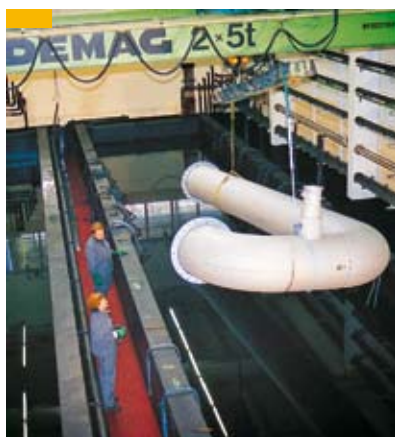
Caption: Full-body pickling of prefabricated castings assures the quality of the pipework system
