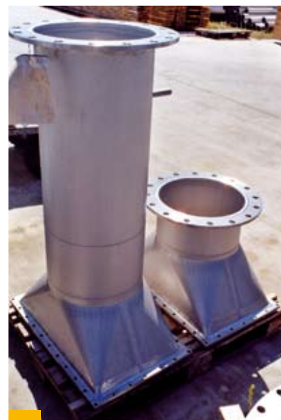
Special components prefabricated to isometric drawings
