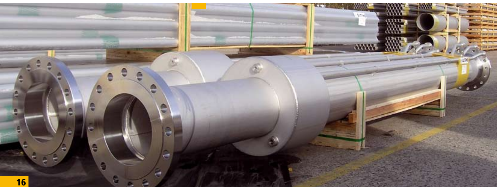
Symbiosis between traditions craftsmanship and modern engineering knowledge: cooler-riser for well construction
