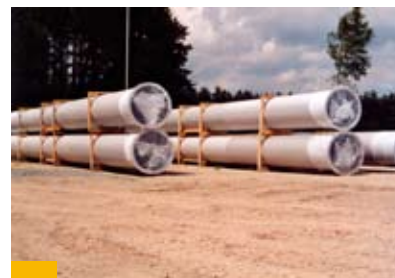
Pipes in 18 m lengths with welded flange in material 1.4571/TP 316L for a water treatment plant in Amsterdam/NL
