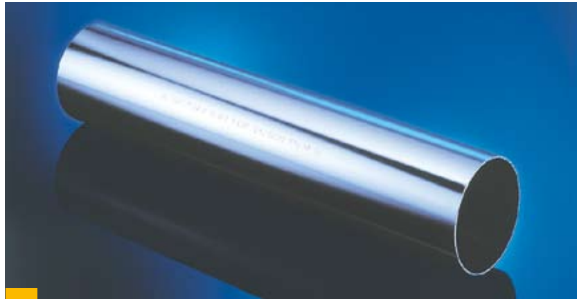
III. 25: Metallic bright surface finish
