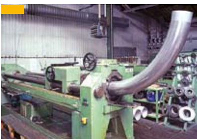
III. 8: Production of a long radius elbow
