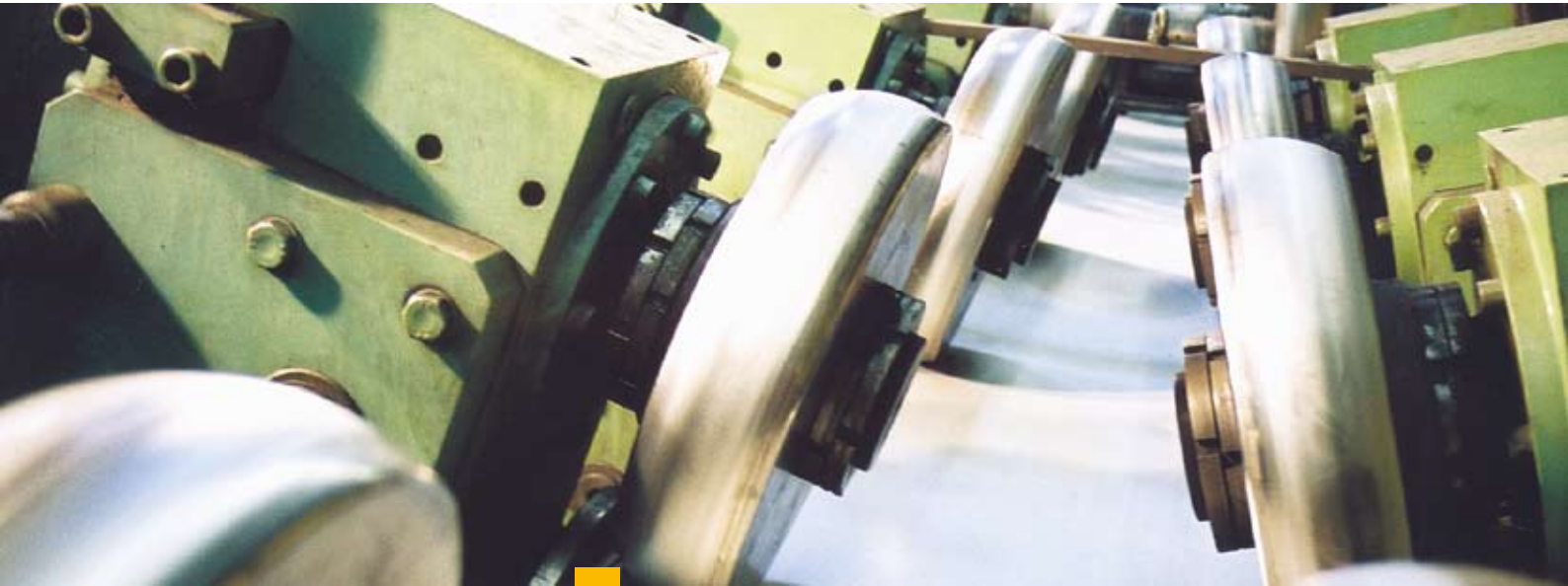
III. 7: Forming from a coil
