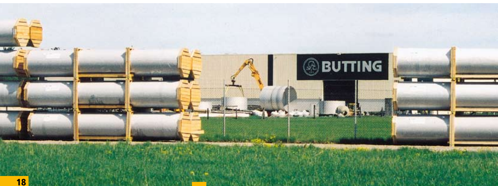
III. 37: Pipes in TP 316L packed in type BK07 – wooden caps, shrink-wrapped
