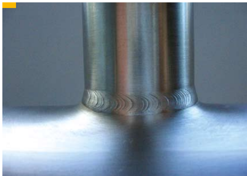
III. 17: Orbital weld of excellent quality
