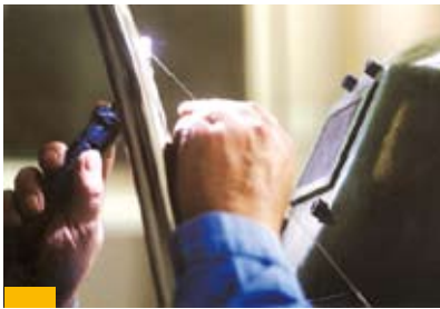
III. 16: Manual welding of a piping component
