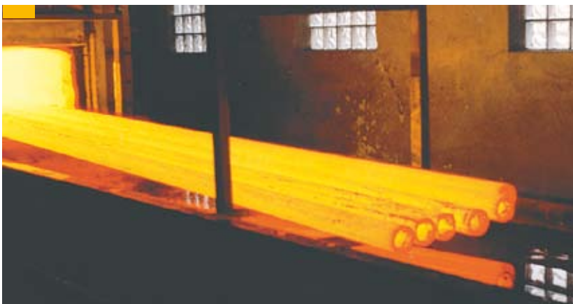
III. 20: Water quench of 6 m pipes after heat treatment
