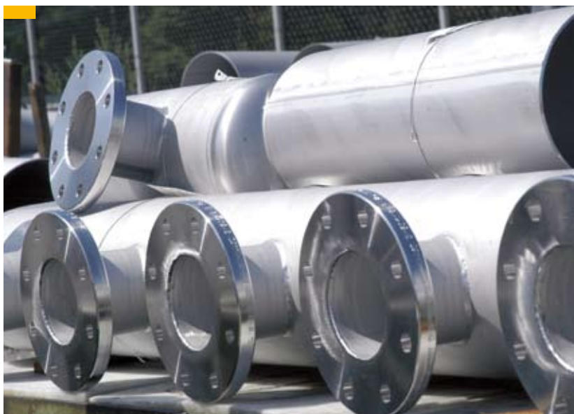
III. 5: Prefabricated piping components made from duplex steel for the ship-building industry
