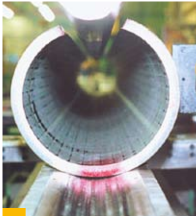
III. 2: Forming of a plate
