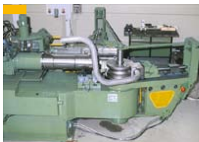
III. 9: Production of integrated bends according to isometric drawings
