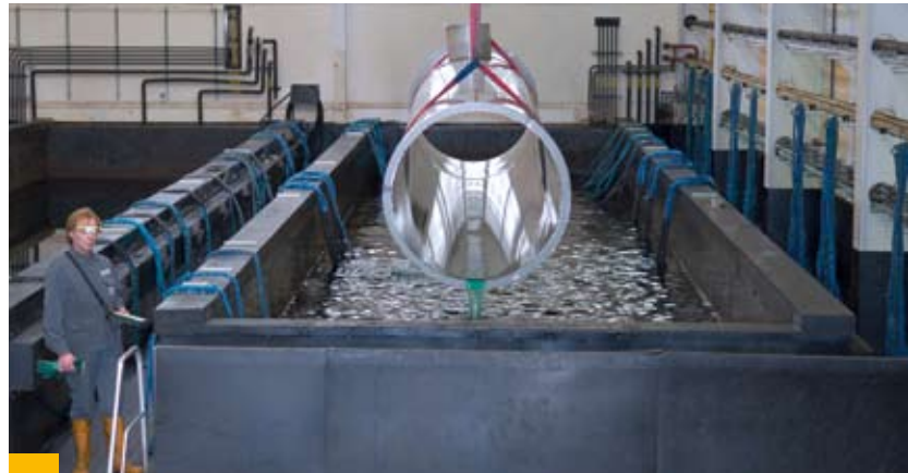
III. 31: Full-body pickling – an economically and environmentally sound surface treatment
