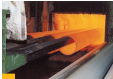
Heat treatment of a thick-walled pipe
