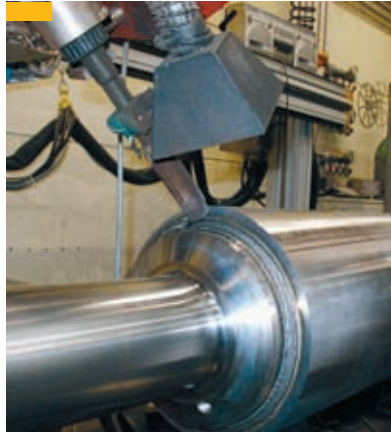
Welding on cones
