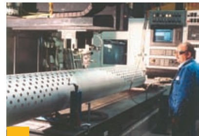
Laser cut-outs created using modern technology and designed for filter pipes
