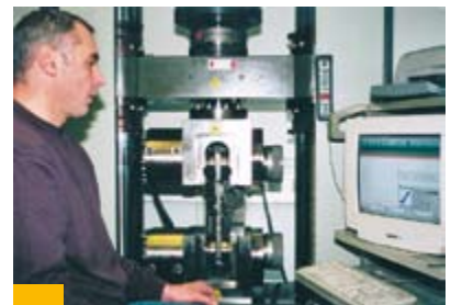
Tensile test with microstrain measurement
