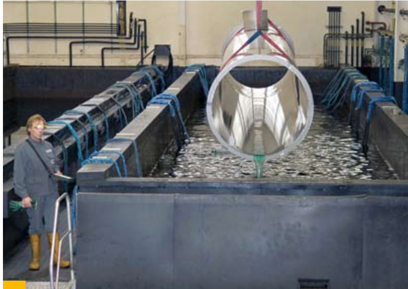
BUTTING full-body pickling – an economical and environmentally sound treatment for surfaces
