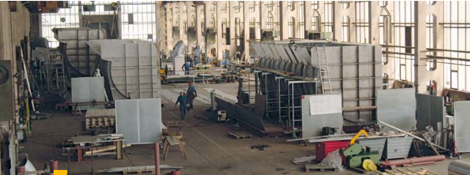
Pulper construction in a manufacturing hall of BUTTING Behälterbau (vessel construction)
