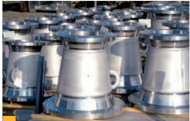
III. 4.2.2_2: Waste gas end pieces for a chemical tanker ready for installation
