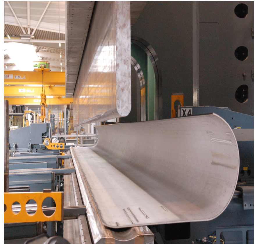
Fig. 1.1.1_1: Production possibilities for pipes from plate (without considering production with optional circumferential welds)
